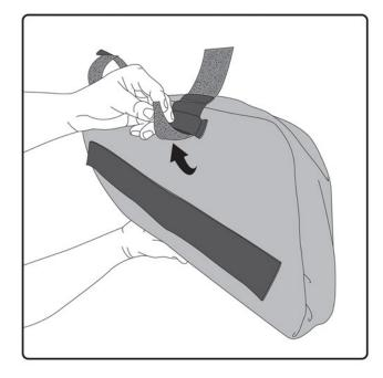
1a) If using Polaris part number 2879509 or RZR4 #2879942 optional lower doors installed pass the middle top strap on bag through the webbing loop on backside first. Then hold bag up to the bottom of the lower frame of the factory door. Pass the 2 upper straps around the door frame and connect the self-fastening straps.
